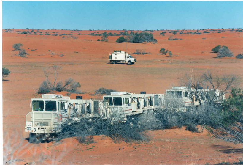
Figure 3-4: Vibrators & recorder truck
