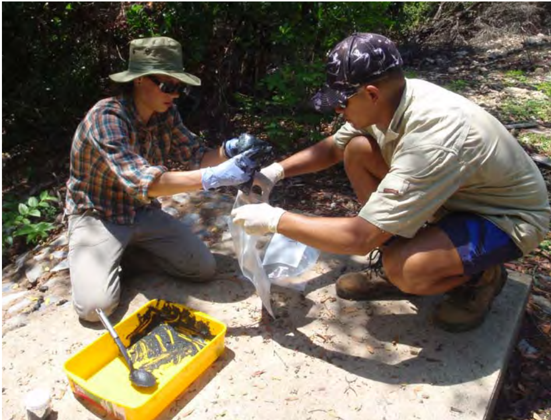
Sampling sediment for assessing pollutant content near the Leanyer-Sanderson sewage treatment plant outfall. Photo: Julia Fortune
