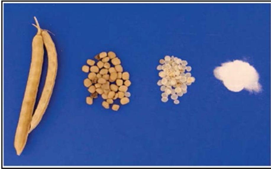
Figure 3-15 Guar gum in its native form, seed form, splits and powder. (Economides and Martin, 2007).
