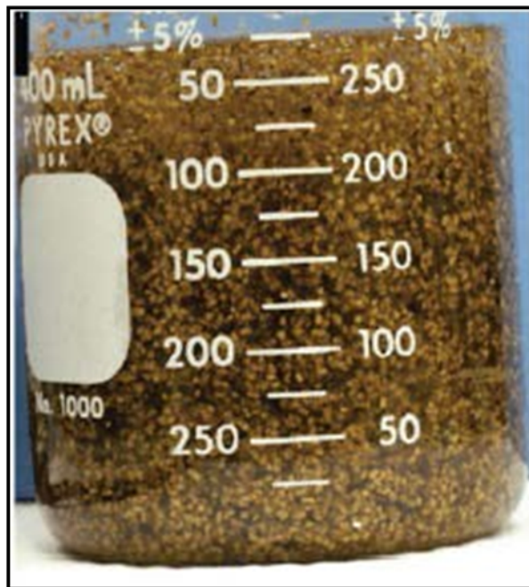
Figure 3-16 Typical sand and guar gum fluid mix. (Source Economides and Martin, 2007)
