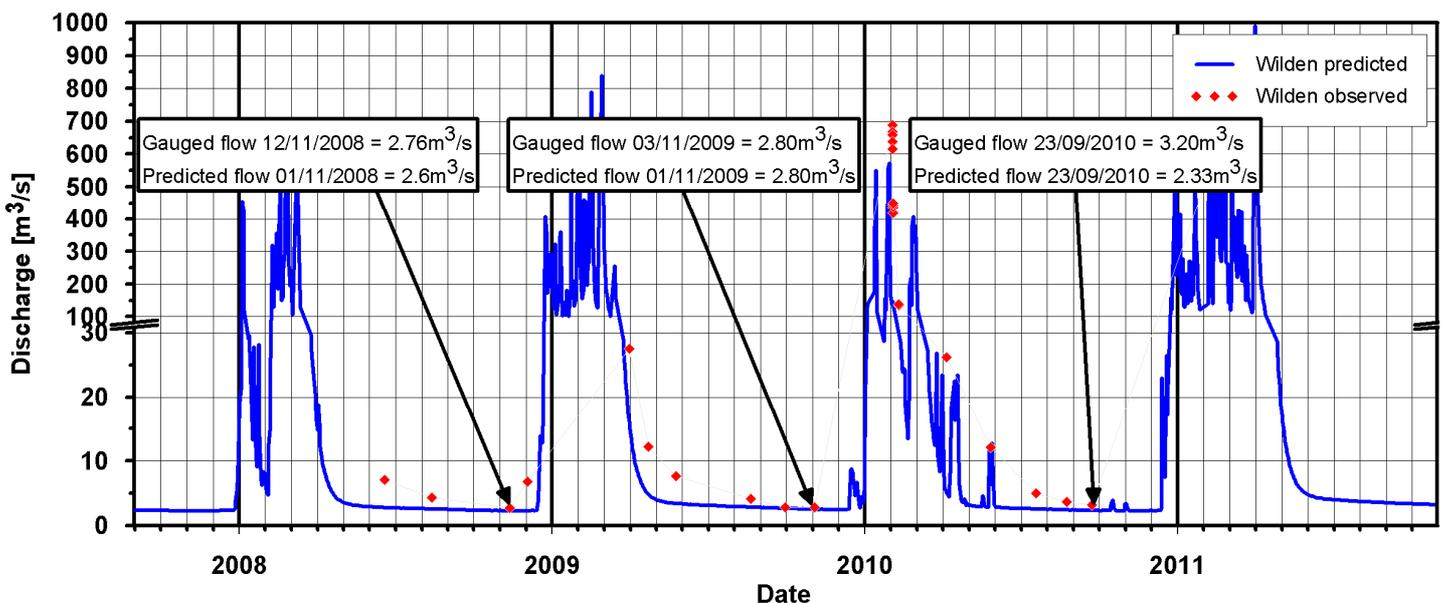
Figure 2: Observed and predicted discharge of the Katherine River at Wilden Gauging Station from mid 2007 to mid 2011.
