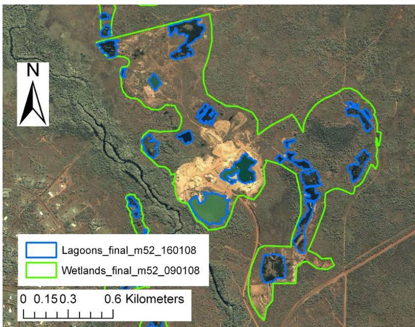
**Figure 4:** The lagoon complex ‘Howard River 5’ as an example for a mixed wetland complex containing natural and man-made water bodies. The man-made water bodies in this complex are sand quarries.
