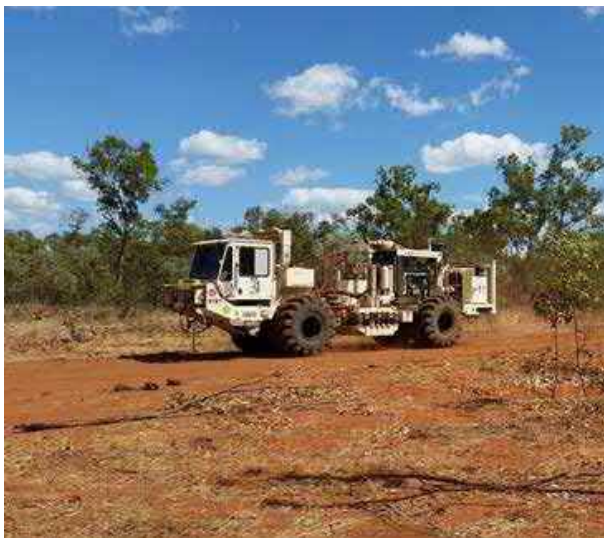
Plate 2 Inova AHV-IV "Renegade" seismic vibrator
