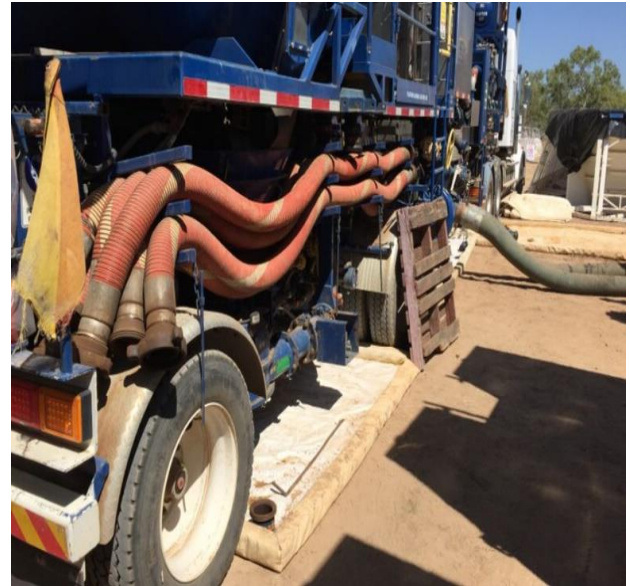
Figure 29: Example of spill mats used to contain drilling additives and under a high-pressure pumping unit.
