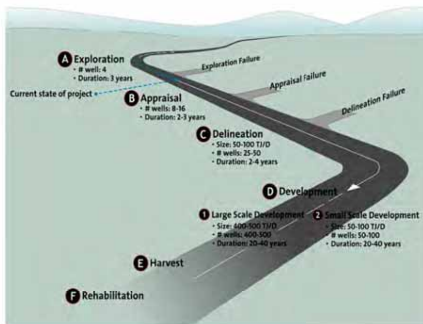
Figure 4 Conceptual Beetaloo Basin project pathway from exploration to development
