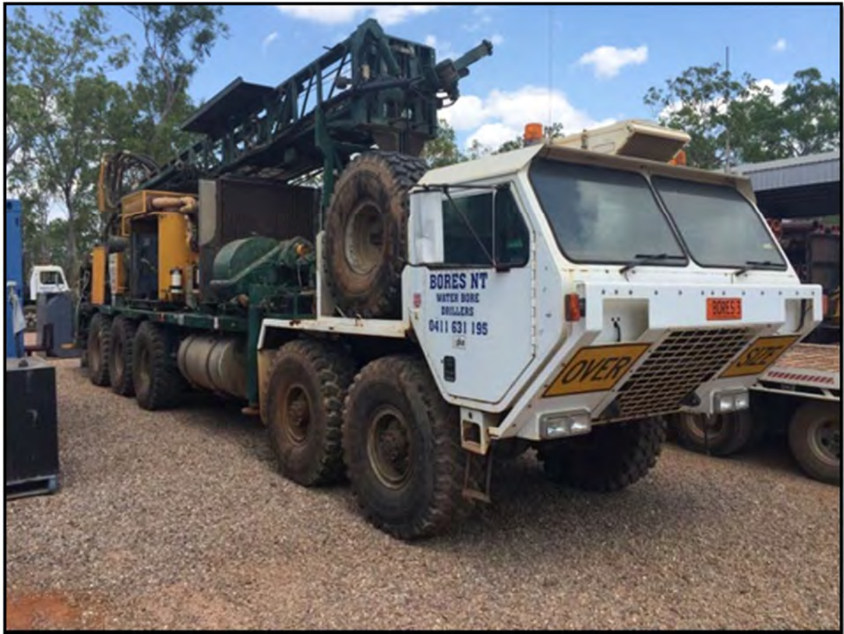
Figure 3-4 An all-terrain type water bore drilling rig
