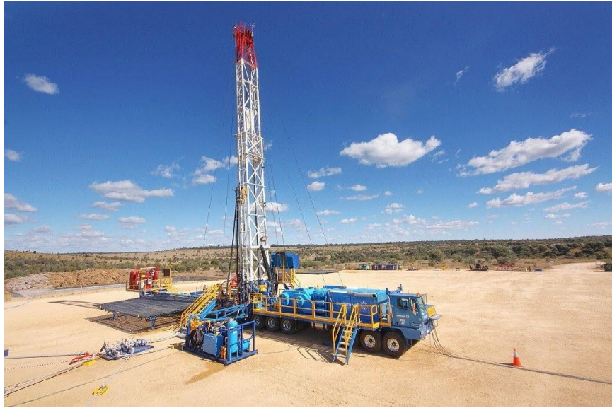
Figure 4-3 Example of a typical workover rig
