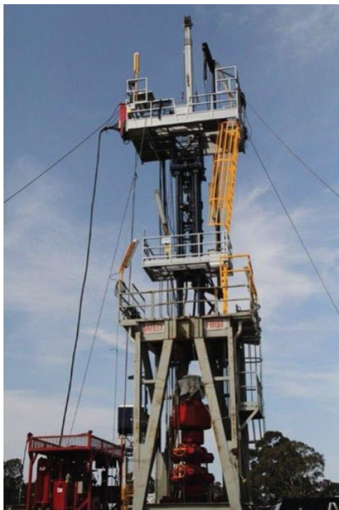
Figure 4-4 Example of a typical snubbing unit (picture, left and schematic, right)
