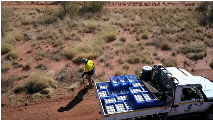
Figure: Seismic line crew deploying geophones
