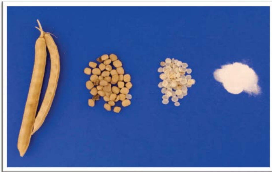
Figure: Example of a typical slurry gum constituent, guar gum – illustrating its native form, seed form, splits and powder.
