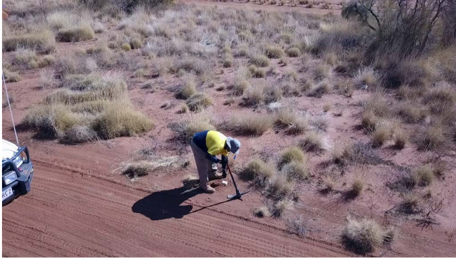
Figure: Seismic line crew planting geophones
