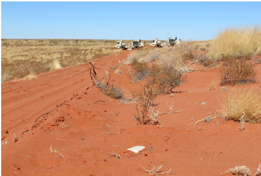
Figure: Geophone planted in the ground
