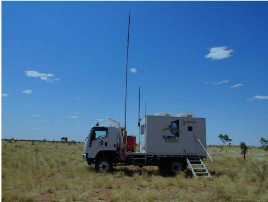
Figure: Seismic Recording Truck
